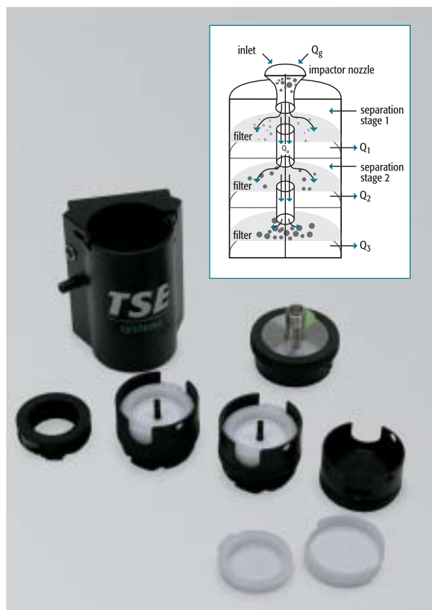
■ OptoPan, a virtual impactor and sketch of the working principle
