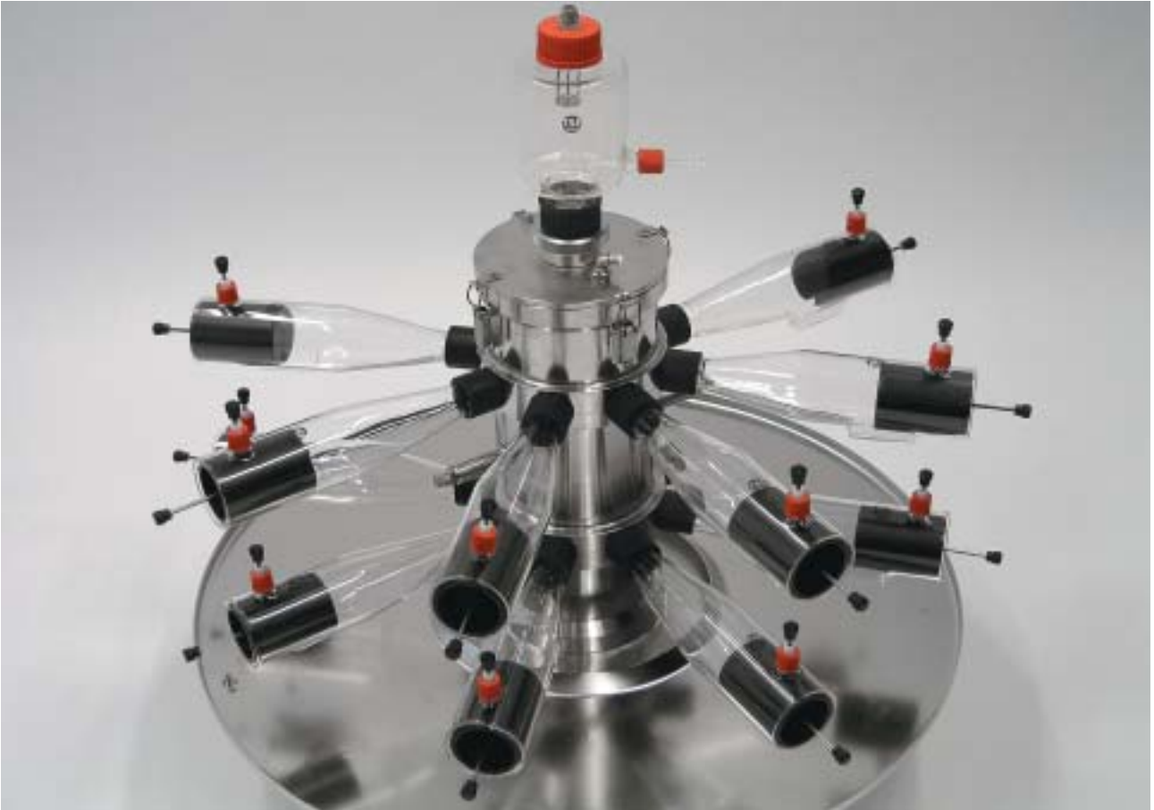
■ Head Nose Only Unit made of stainless steel with glass restrainers and mixing device with impactor plate for dust aerosols
