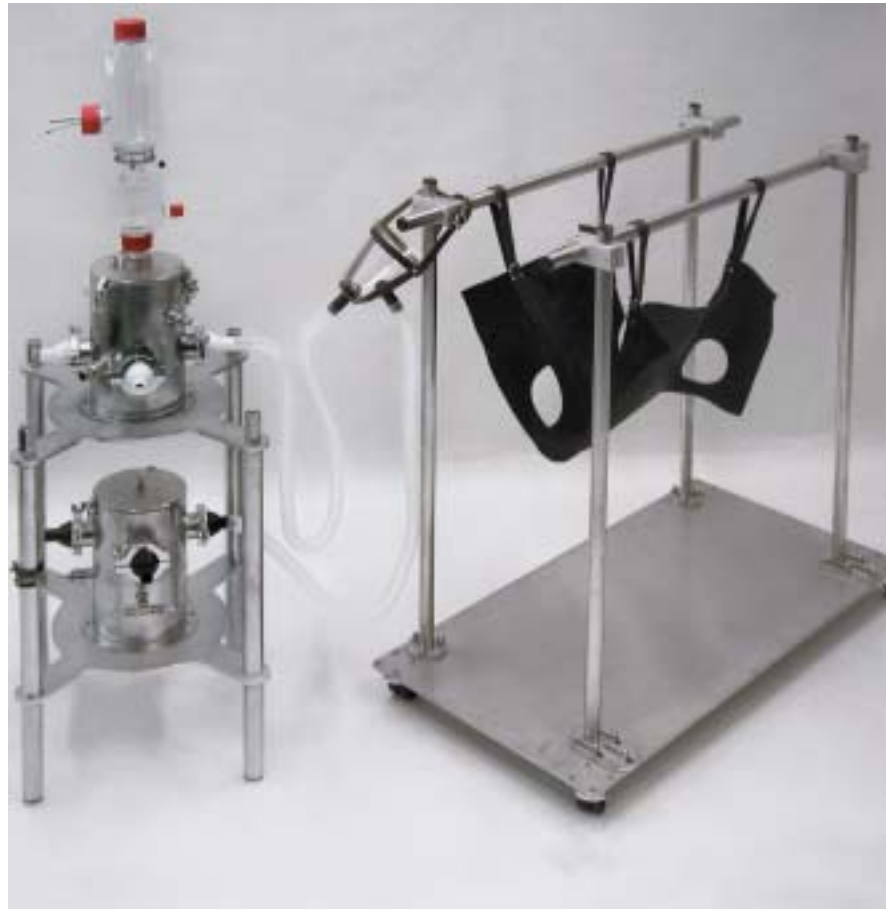
■ A Dog Exposure Unit for the application of liquid aerosols with inhalation mask, holding device and leather harness for the dog
