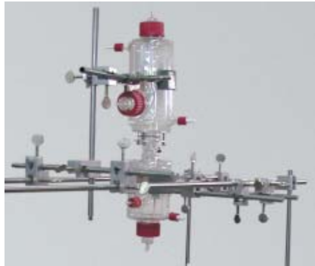
■ Water-jacketed mixing units for aerosol conditioning
