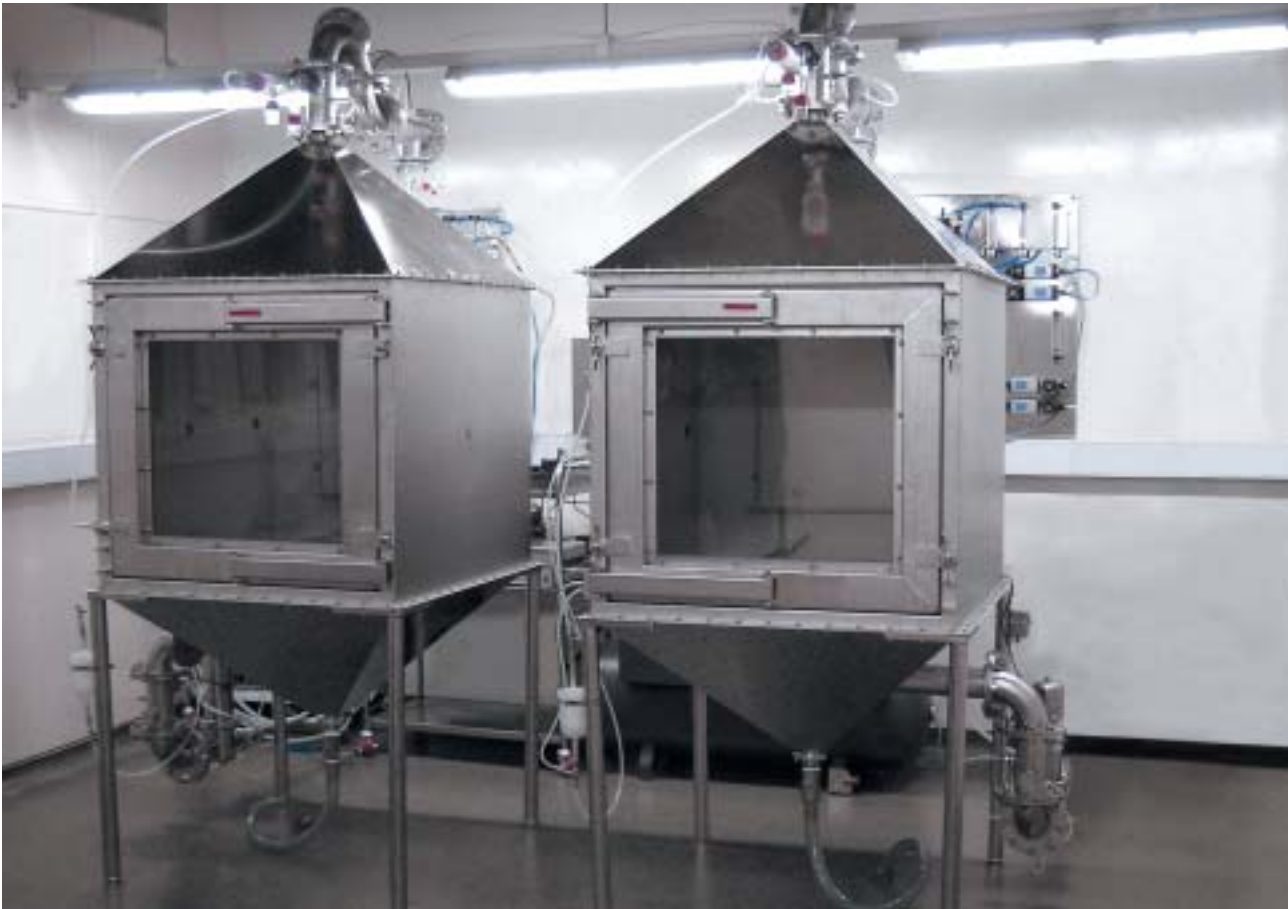
■ Whole Body Units with aerosol conditioning and exhaust air line – in the background a mounting panel with flow control units
