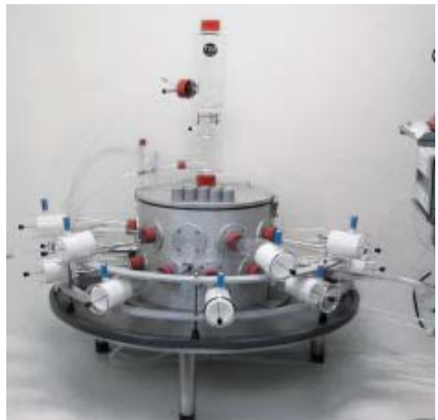
■ Head Nose Only Unit in fume cupboard with mounting panel
